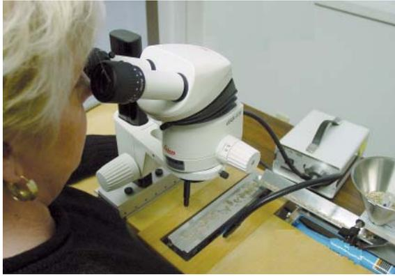
Figure 3. The EVS being used where the analyst sits in an ergonomically correct position and uses both eyes at optimum magnification. The seeds flow continuously and the process can be started and stopped any time to remove contaminants.
