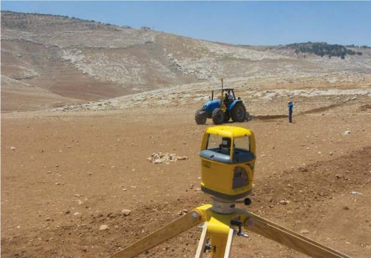
*Laser guidance system for tractors: this innovation has greatly increased the speed and accuracy of preparing contour ridges*
