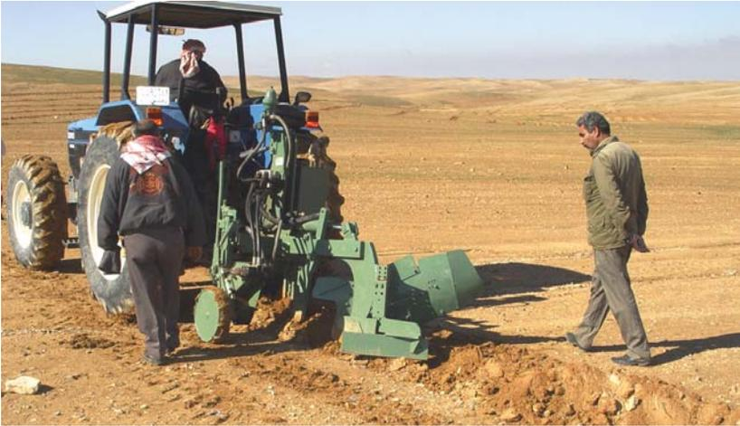
*The Vallerani plow has mechanized the process of building water harvesting structures and rehabilitating degraded rangeland*
