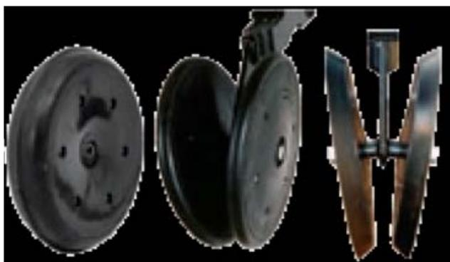
*Figure 7. Types of press wheels for no-tillage drills*
